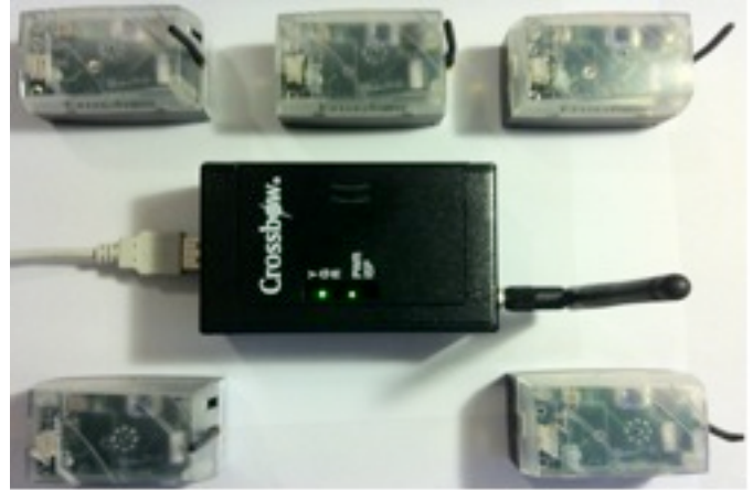
Fig. 1. Crossbow Platform, BaseStation (BS) and sensors.
