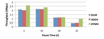
Fig. 2: The throughput for the different routing protocols.
