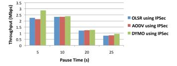
Fig. 6: The throughput for the different routing protocols using IPSec.
