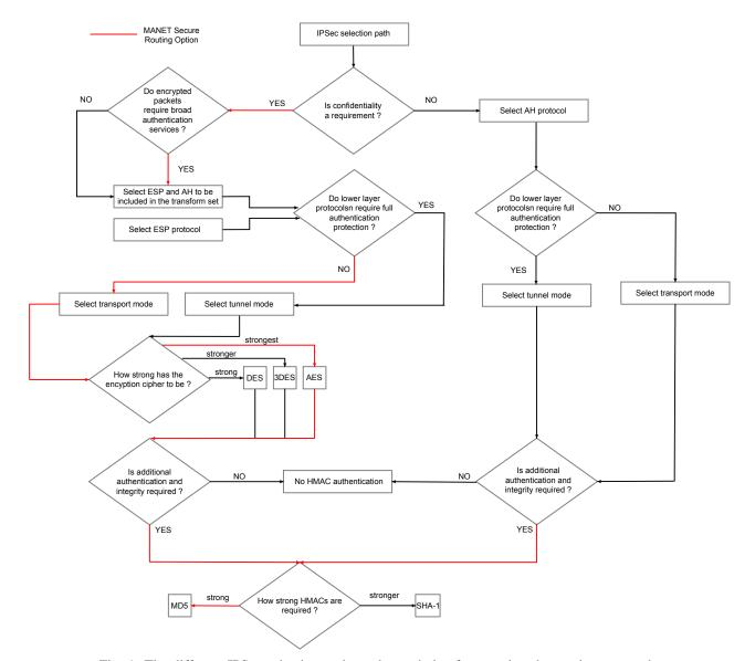
Fig. 1: The different IPSec selection paths and our choice for securing the routing protocols.
