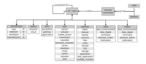
Fig. 1. Conceptual model of APPARATUS in Entity-Relationship Diagram
