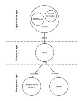
Fig. 3. Temperature monitoring application layout
